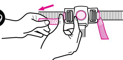
Use slide adjuster at waist for tighter adjustment.
